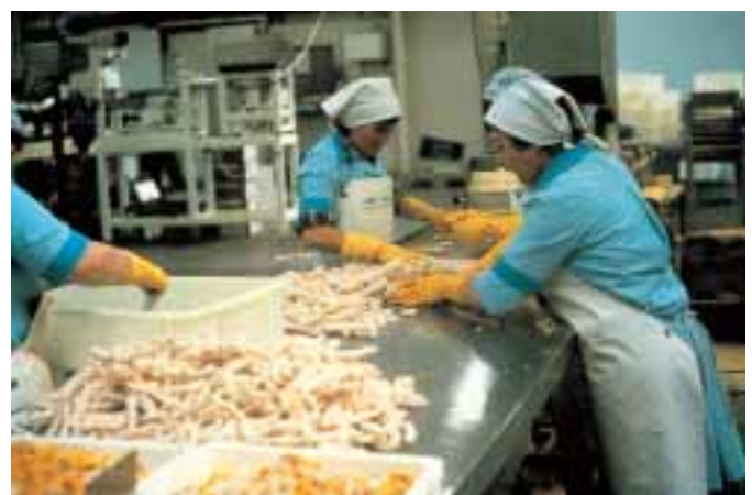
A cluster of wheezing and rhinitis occurred on this prawn processing line. High pressure hoses (used to free the prawns from the shells) had created aerosols containing crustacean protein
